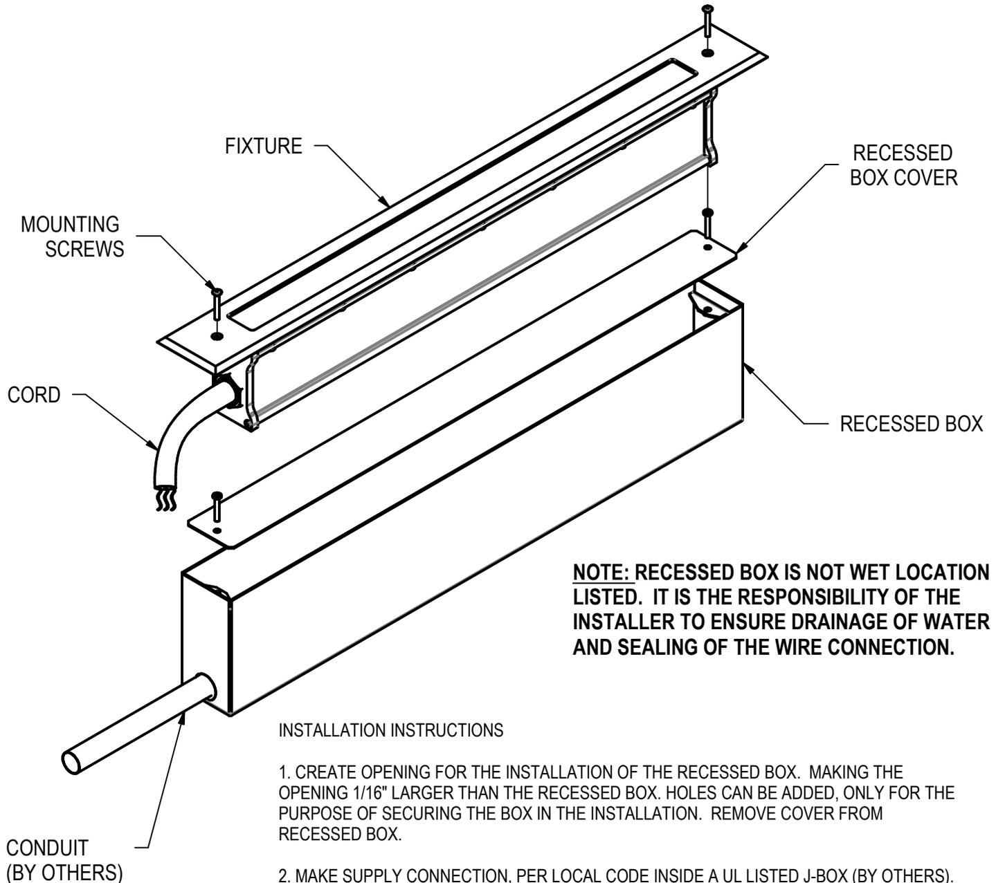
**NOTE: RECESSED BOX IS NOT WET LOCATION LISTED. IT IS THE RESPONSIBILITY OF THE INSTALLER TO ENSURE DRAINAGE OF WATER AND SEALING OF THE WIRE CONNECTION.**
